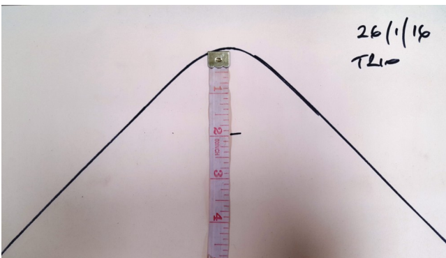
Fig 6: Measure and mark 2 inches down from the apex.
