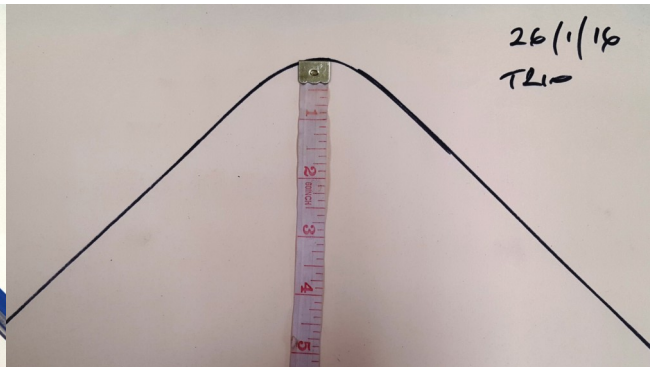
Fig 5: Remove Flex Curve Ruler and place a tape measure or ruler (with inches on it) as shown here.
